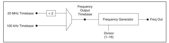
Figure 7-26. Frequency Generator Block Diagram
